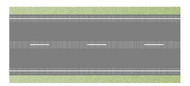
Figure 4: Rumble road surface along centre line and edge lines. The width of vehicle lanes decrease with decreasing speed limit by increasing the width of the rumbling surface.
