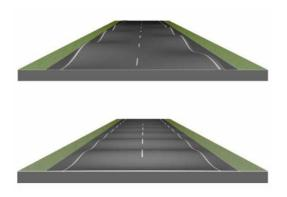
Figure 2: Rocking and waving road surfaces
