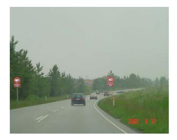
Figure 13: Variable speed sign is activated when crossing traffic approach
