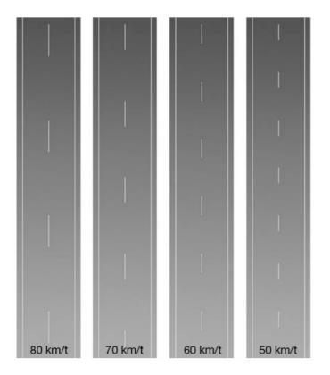
Figure 1: Length and spacing of centre lines depends on speed limit
