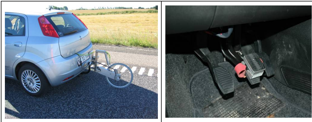
Figure 2.1 Test car with fitted measurement wheel and pressure meter on brake pedal.
