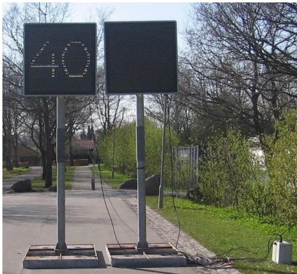
Figure 4: Two VMS's on loan from the Danish Road Directorate. Only one was used.
