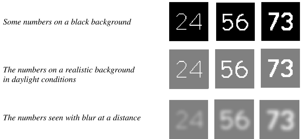
Figure 11: Legends are seen with a reduced contrasts depending on the stroke width.
