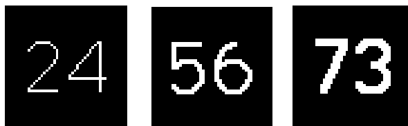
Figure 25: Legends with a height of 20 pixels height and stroke widths of 1, 2 or 3 pixels.
