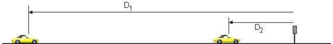
Figure B.4: Two distances defining a range in which reading can proceed.
