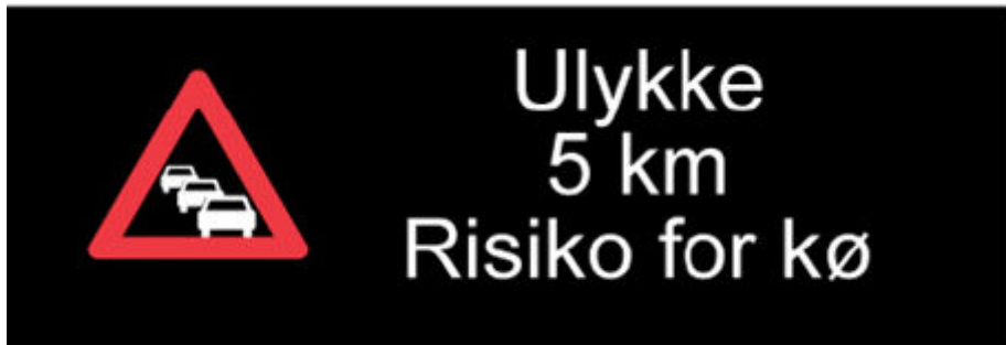
Figure B.5: Illustration of a VMS with three text lines and a warning sign.
