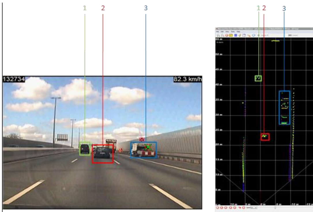
Figure 2 Example: Screen dump photo from the scene camera (left) and the laser scan result (right) from the same traffic situation. The small green cross with the red ring around it on the photo indicates the eye glance direction of the test driver.
