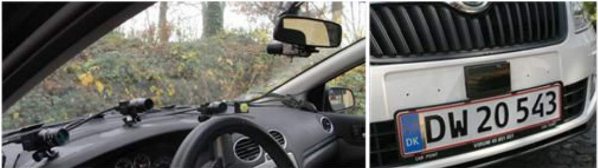
Figure 1 The 3-camera system for tracking eye movements together with the scene camera behind the rear view mirror (photo left). The scanner is installed in front of the car (photo right).
