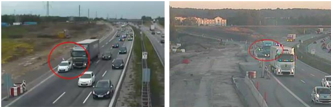
10 11 12 Figure 6 The car drivers in both accidents do not accelerate sufficient enough on the slip road to 13 pass the truck completely. The truck drivers do not give way even though the cars are ahead of 14 them. Furthermore, the taper is too short in both merge areas.
